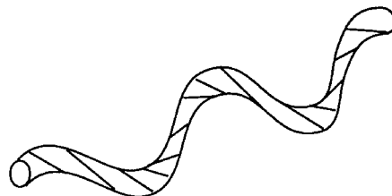
Fig. 2 Departure of the core from a straight line.
